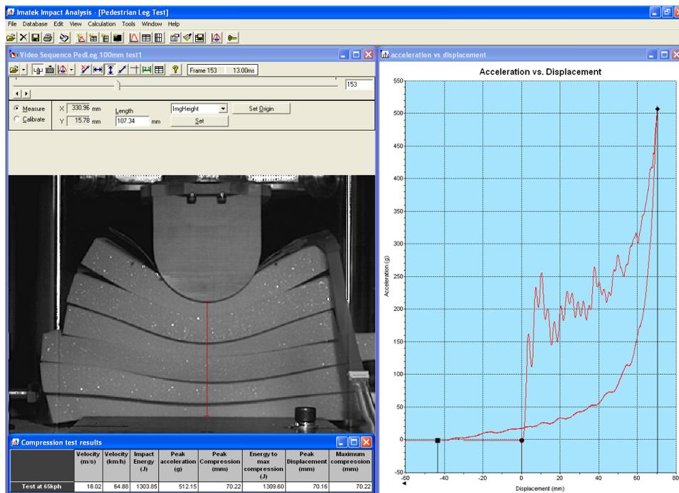
Fig 4 shows layered specimens of polymeric foam. The specimens are undergoing an energy absorption test using a drop weight impact tester fitted with an adult pedestrian leg profile striker. Integrated high speed video enables the compressive characteristics of the specimen to be observed and measured in conjunction with the data captured for energy absorption efficiency.
