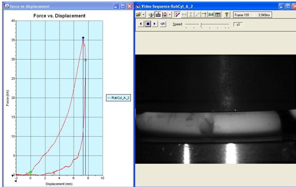
Fig 3 shows a cylindrical specimen of rubber undergoing a high-rate compression test in a drop weight impact tester to determine when failure occurs. The specimen is compressed between two flat surfaces at a high rate, typically 10m/s, to achieve strains of around 80% and peak loads in excess of 35KN. Integrated high speed video enables the point at which catastrophic failure of the specimen occurs, in this case during elastic recovery and after the specimen has achieved peak compression.
