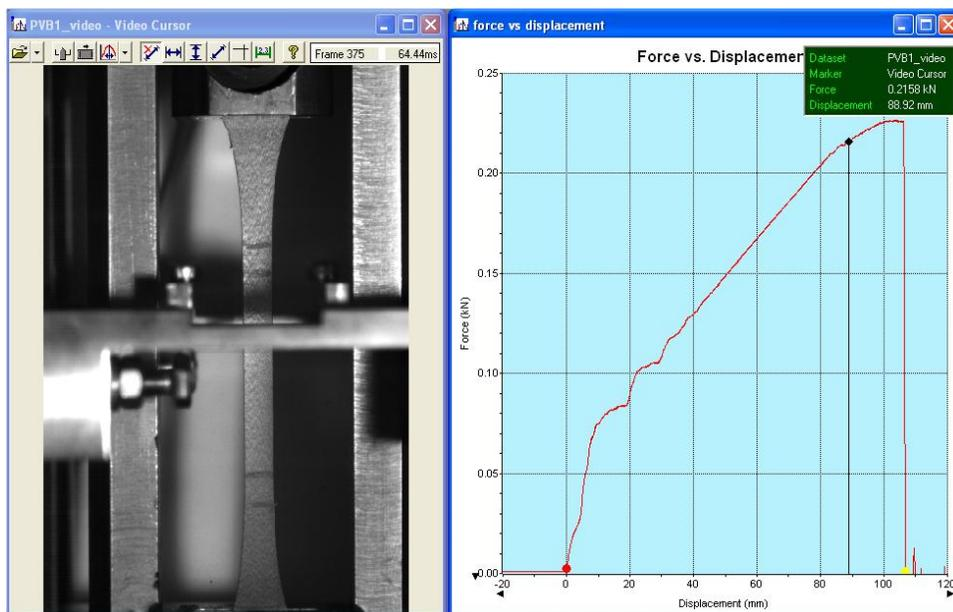
Fig 2 shows a specimen of PVB (poly vinyl butyral), commonly used as an interlayer for laminated glass, particularly car windscreens. The specimen is undergoing a high-rate tensile test in a drop weight impact tester. High speed video enables direct measurement of strains exceeding 100%, and also enable the exact mode of failure to be determined - in this case a slight defect in the sample preparation process led to premature failure.
